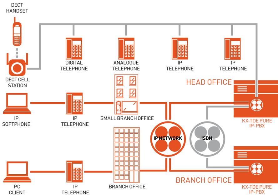
IP network infrastructure, which already exists in the majority of companies, can now carry voice along with data. Designed to support convergence through a modular structure, the system allows a harmonious migration towards VoIP, allowing voice and data communication to work within the same network.
